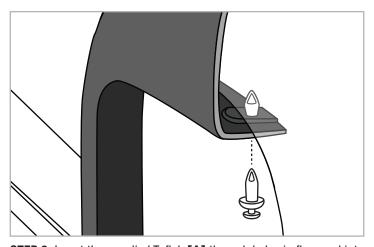
**STEP 3:** Insert the supplied Tuflok **[A]** through holes in flare and into vehicle's factory holes.
