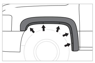
STEP 2: Starting at the top center, install 6 supplied Tufloks.
