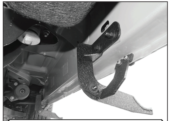
(Fig 15) Passenger/right center Brackets installed
