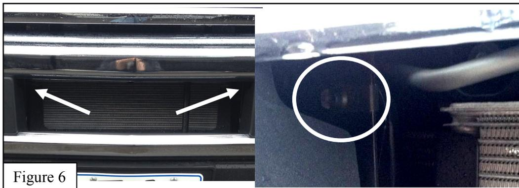
8. Slide grille behind bumper from the top side and insert grille in to bumper opening. refer to **Figure 7**.
