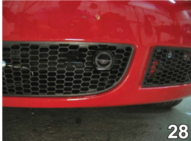
28. Reinstall the fascia and center grille, inserting all screws, pushpins, and bolts. Align the fascia to its original position and, using a diagonal cutter, trim necessary openings in the grille for attachment tabs, convenience links, and electrical rods. The installation of the baseplate is complete.
