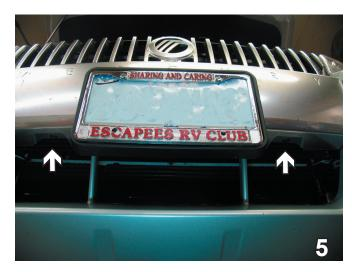
5. Under the front of fascia, remove a Phillips pushpin on each side of the license plate. Pull fascia forward to remove. Set pushpins and fascia aside to be reinstalled later.
