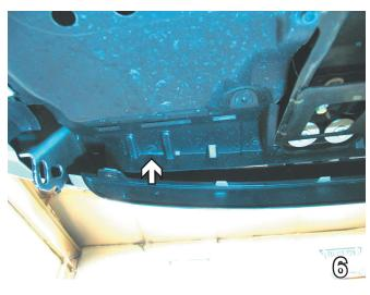
On the front corner of belly pan, use the 10mm socket to remove one metric bolt. Do this to both sides of the vehicle. Set bolts aside to be reinstalled later.
