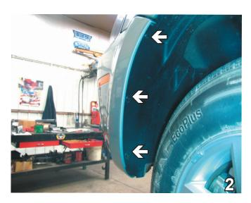
Just forward of the front tire, inside the wheel well, remove three Phillips pushpins. Do this to both sides of the vehicle. Set pushpins aside to be reinstalled later.
