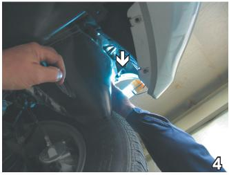
4. Remove one pushpin from bottom corner of fascia. Do this to both sides of the vehicle. Set pushpins aside to be reinstalled later.
