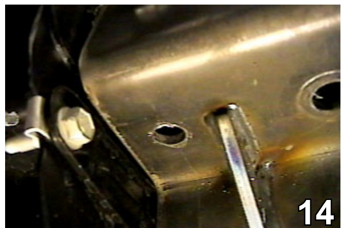
14. Reinstall the metal bumper. Install the baseplate using the 5/8-11x8" hex bolts, 5/8 flat washers, 5/8" lock washers, and the 5/8-11 hex nuts. Using the baseplate as a template, drill the two holes using the 17/32" drill bit. Do this on the side of the frame rail and drill one on the bottom. Do this to both sides of the vehicle.
